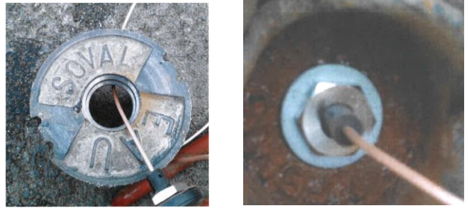
Figure 21. Thread antenna into position and secure in place with supplied nut and a suitable washer
