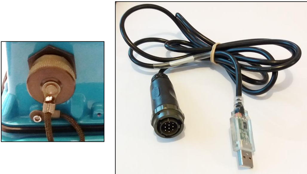
Figure 3. A typical Multilog2 COMMS connector and an example COMMS cable (with USB-A)
