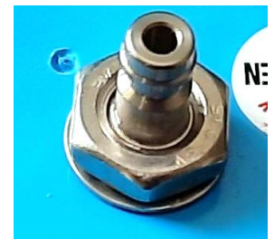
Figure 10. Connection to an internal water pressure transducer
