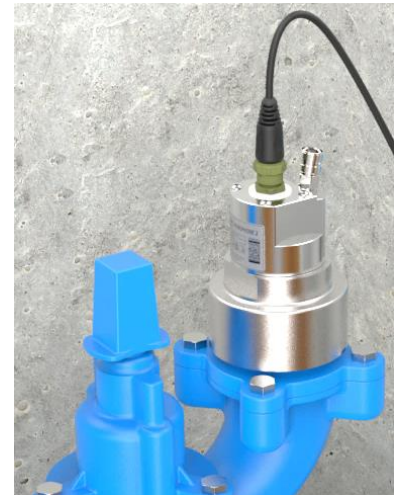
Figure 18. Example of a Hydrophone-2 installation
