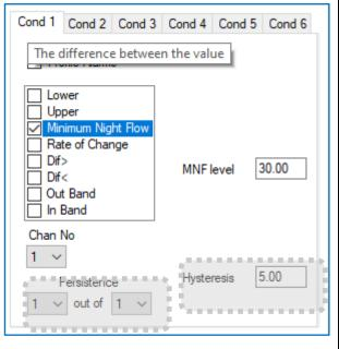
Note: Hysteresis settings have no bearing on the function of this trigger. Persistence settings have no bearing on the function of this trigger.
