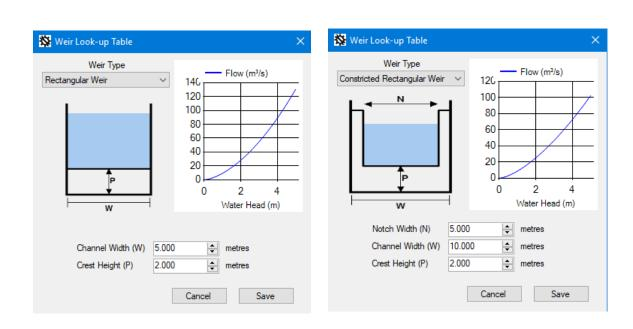
For a weir of a different shape to the above options, but where the "depth to flow" characteristics are known, they can be entered in tabular form.
