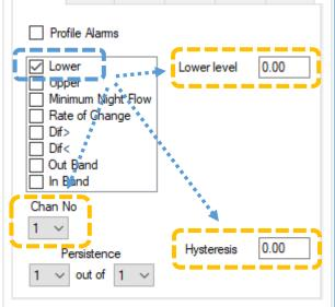
The relevant channel(s) have to be selected within the tab. The channels must have previously been set up and also saved to the logger; if not, they are unavailable for selection.
