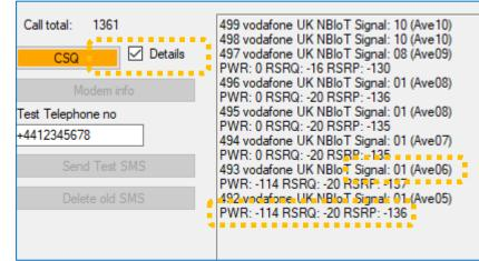
**RSRP value:** The following guidelines are given for the cellular network signal, (as measured with the chamber closed):
