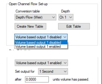
Set the required pulse duration and the number of units of volume required to pass to activate each pulse event.
