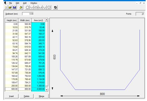
The cross-sectional area table must be saved to the logger using the "Transfer Data" button/icon.
