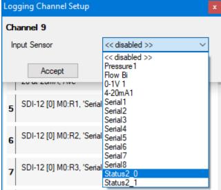
The "\_0" and "\_1" refers to the specific pin being used on the logger interface connector; refer to your logger user-guide for details of pin number or wire-colour of any HWM-supplied cable.
