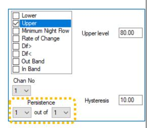
However, if the data from the channel has any possibility of "blips" (spikes or other noise characteristics) the use of the **persistence** settings can be employed to ensure (add greater certainty) that the trigger threshold has been crossed. This is, however, at the expense of delaying the alarm message; it is the nature of the assessment process.
