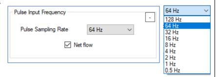
Ensure the logger can capture pulses that are generated at the *maximum* expected meter output rate.
