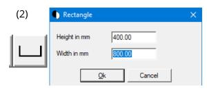
completed from the shape and dimensions. It can be further adjusted by inserting lines or deleting lines from the table. The cells with height and width data can be edited. A sediment depth can be added to reduce the area. The cross-sectional area
